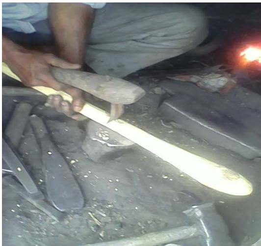
A suitable wooden handle being marked out
