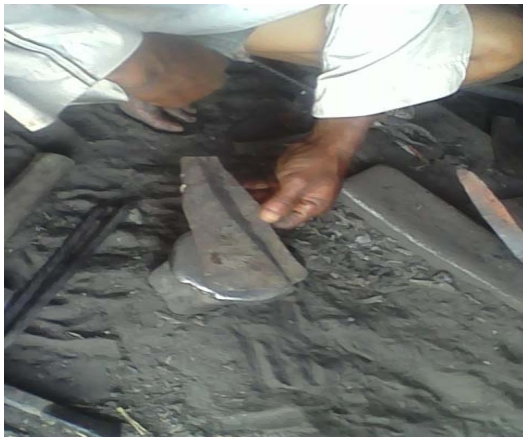
The intended shape and size of the implement is marked out on a scrap
