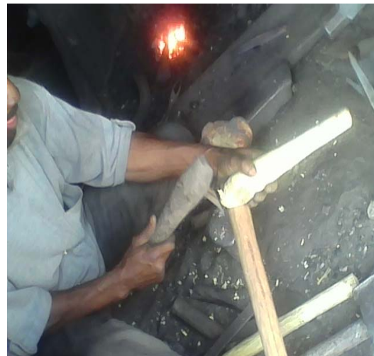
Trimming of the handle
