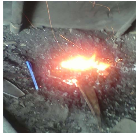
The scrap is then heated in the fire ember
