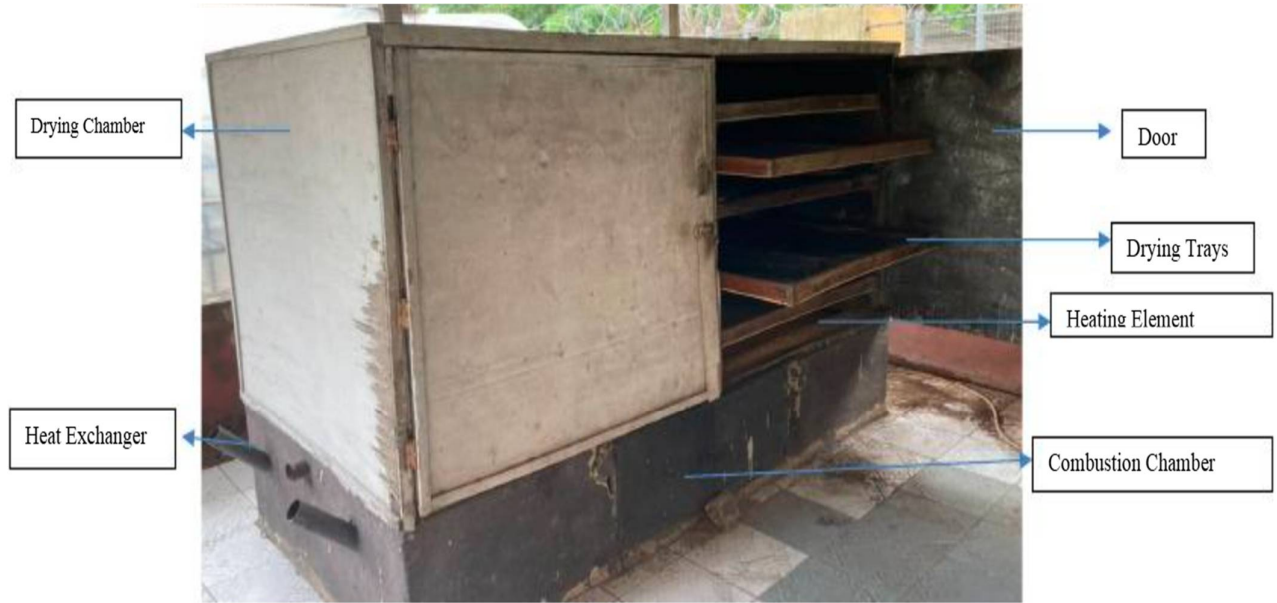
Figure 1: NSPRI-Multi Crop Dryer
